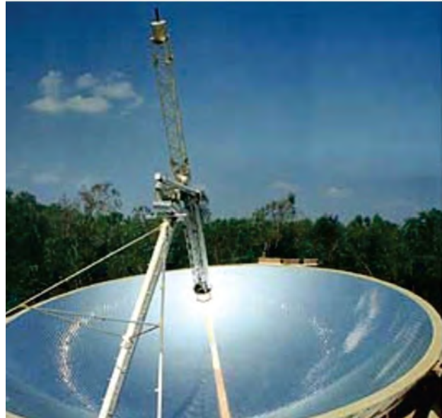
Solar Parabolic Concentrator with south orientation
